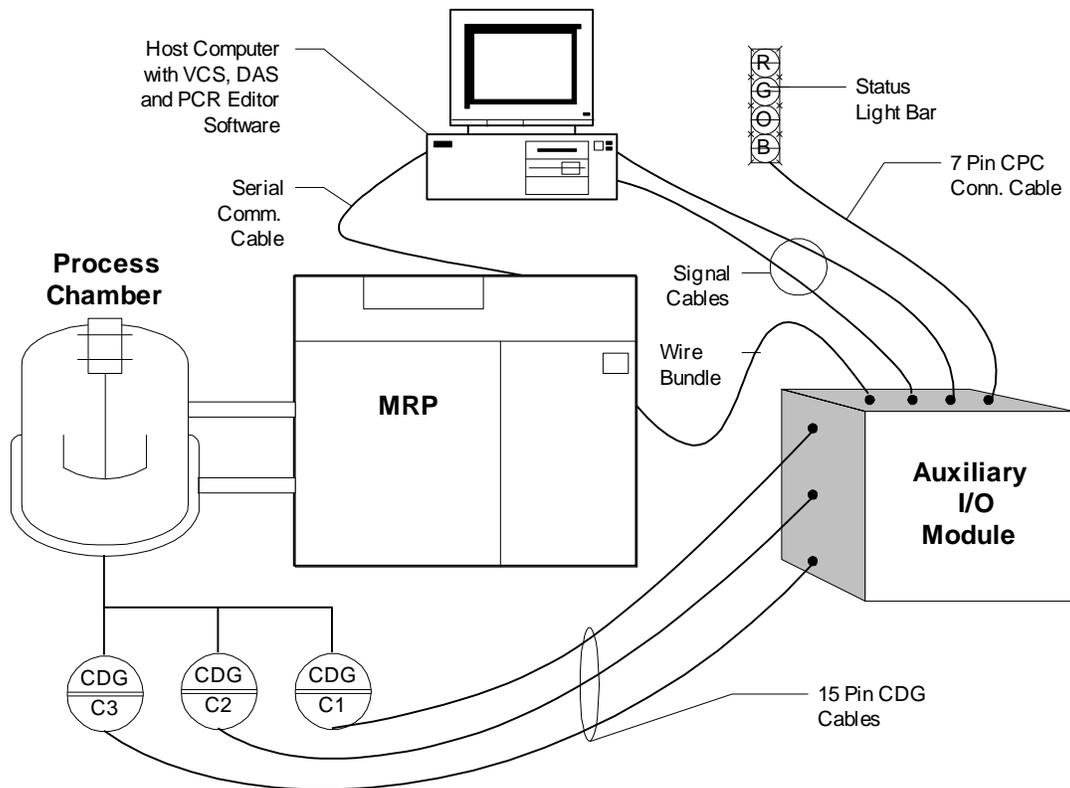
Figure 2 - 2 HGRS System Components
